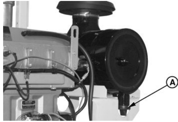
Rubber Dust Unloader Valve
